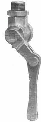
Fig. 37 Emergency brake cock
